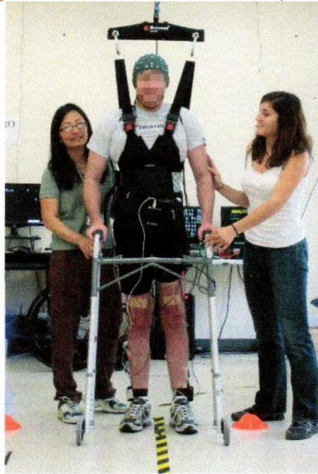
A BCI system allows a man whose legs had been paralyzed to walk without robotic support (credit: courtesy of UCI's Brain Computer Interface Lab)
